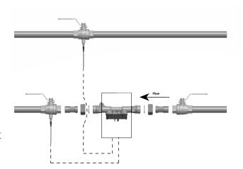
Figure 3: Integration with ball valve (recommended up to and including DN 25)
